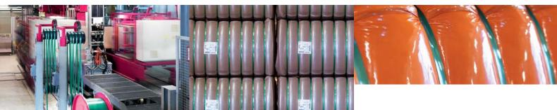
Optimisation for higher efficiency: a 500 tonne ball press was converted by TITAN to strap fibre balls using PET Straps. The facility is equipped with two strapping heads from the VK 10 K-120 19B series. It offers the option of building in additional aggregates.
