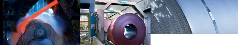
For this range of applications it often gets very hot, especially in the steel industry: temperatures which can be up to 900 degrees Celsius even in the packaging areas require special strapping solutions. TITAN has been the leader in this field for ages. Tailor-made solutions for hot-strapping steel coils offer the highest security even under extreme weight and temperature conditions.
