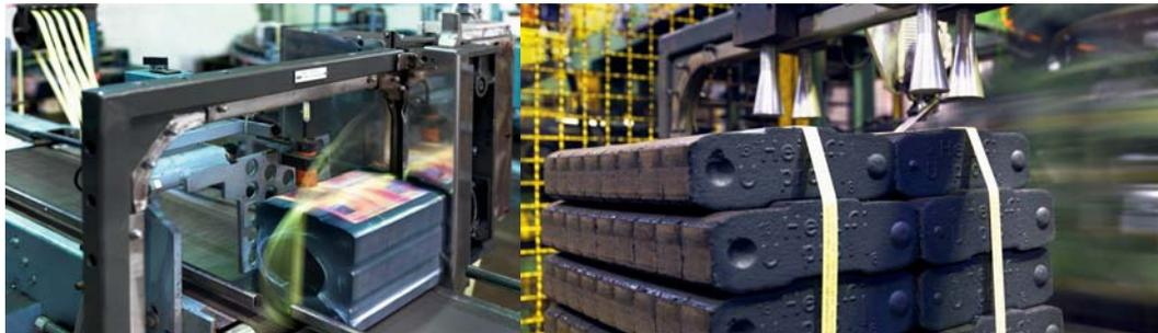
When making briquettes brown coal is chipped, dried and pressed with a pressure of about 1000 bar. The dusty production environment and the special characteristics of the end product place high demands on the strapping and packaging technology.
