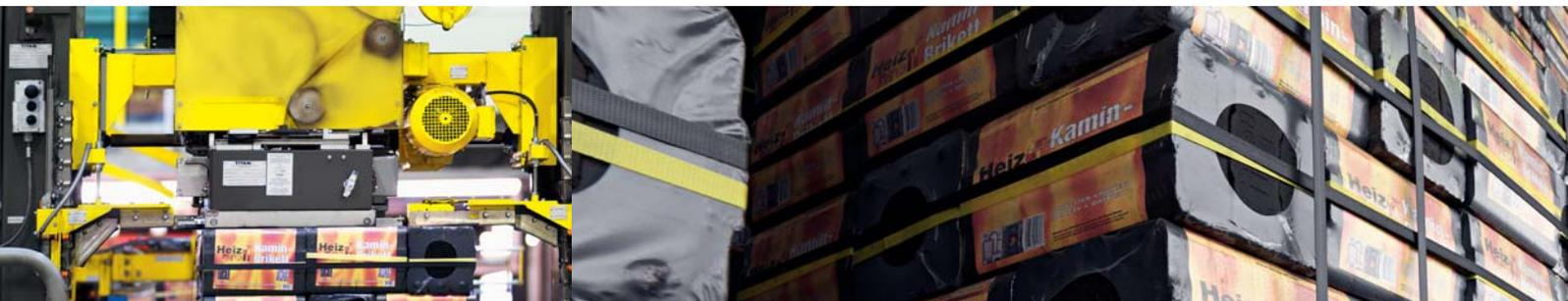
Briquette pallets are strapped with a weight between 10 and 25 kilograms. As a plus for the end consumer the packaging band for the 10 kilogram packages also serves as a carry handle. The 25 kilogram briquette pallet can be stacked for storage and is wrapped with cling-film before being horizontally and vertically strapped.
