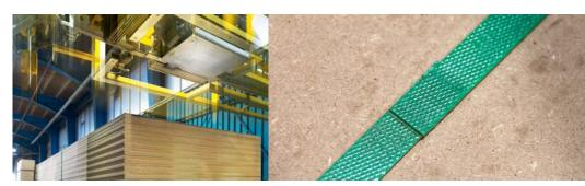
Extremely high and permanent sealing quality: the VK 10-O PET strapping machine secures plywood and MDF sheets with the TITAN thermo-weld seal. The facility automatically feeds squared wood under the sheeting package from a mobile 10 slot magazine.
