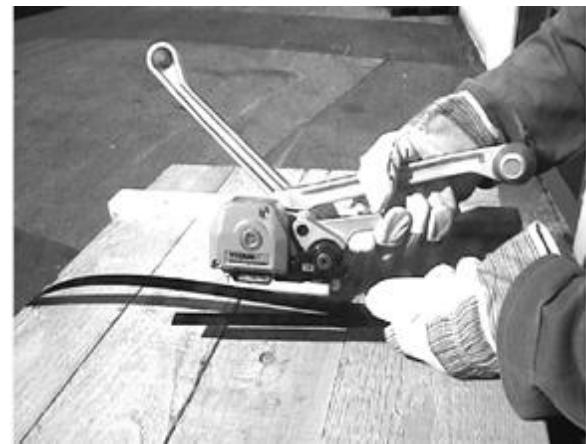
With the left hand hold the upper and lower run of the strap together. Both straps must be placed exactly on top of one another. Grip and press rocker **520** together with the cutting lever **96** with the right hand. Insert the steel strap laterally until it strikes against the case wall, ensuring that the lower run of strap projects slightly out of the tool at the front. The right hand now releases the levers which have been pressed together.
