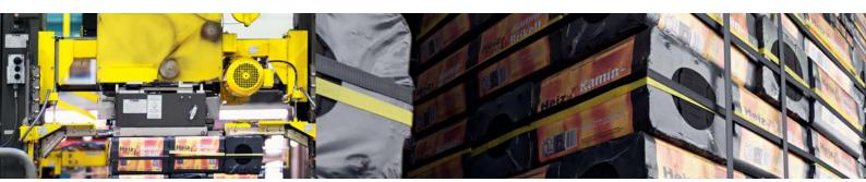
Briquette pallets are strapped with a weight between 10 and 25 kilograms. As a plus for the end consumer the packaging band for the 10 kilogram packages also serves as a carry handle. The 25 kilogram briquette pallet can be stacked for storage and is wrapped with cling-film before being horizontally and vertically strapped.
