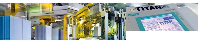
Transport securing for sand lime bricks is a real challenge for strapping technology. The high weight and the sensitive surfaces and edges of the stone demand flexible stabilisation during storage and transport.
