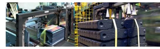
When making briquettes brown coal is chipped, dried and pressed with a pressure of about 1000 bar. The dusty production environment and the special characteristics of the end product place high demands on the strapping and packaging technology.
