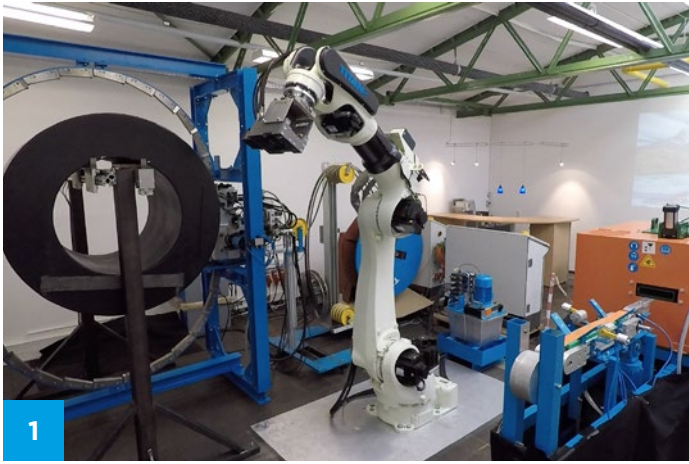
The robot is in the parking position and waits for the signal that a coil is ready.
