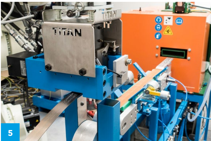
The strap is deposited on the conveyor belt.
