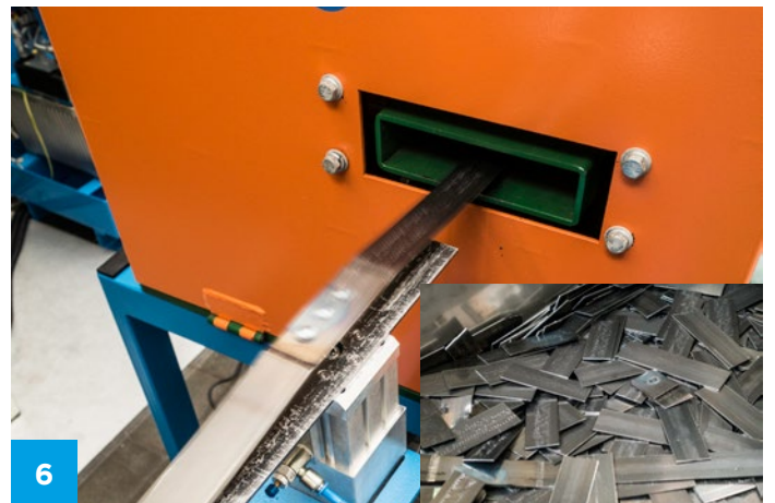
The strap runs into the chopper and is cut into pieces.
