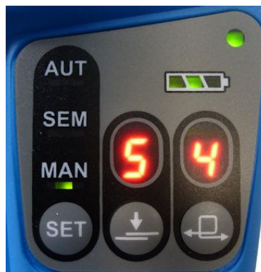
Li- Ion storage battery half-full
