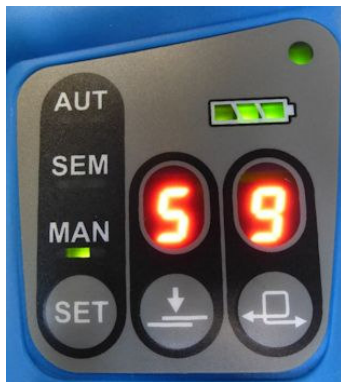
Li-Ion storage battery fully charged
